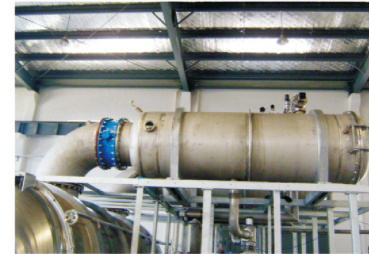
外置式多冷阱交替捕水 External multi-cold trap alternate condensing
